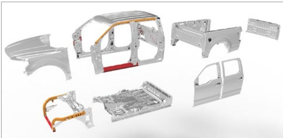
Every component seen in the image of the 2015 F-150 above is made of high-strength, military-grade aluminum alloy. The orange-colored parts are hydroformed aluminum, with the roof rails creating a cage-like structure around the doors. The red-colored rocker panel—seen here on Super Crew Cab—is an extrusion, which provides increased lower-body strength.
